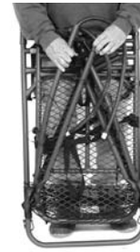
FIGURE 13 CLOSE SPREADER ARMS OVER STAND- ING PLATFORM
