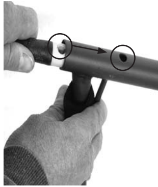
FIGURE 2 INSERT CABLE ASSEMBLY INTO SPREADER ARMS (LINE-UP SPREADER ARM AND CABLE HOLES)
