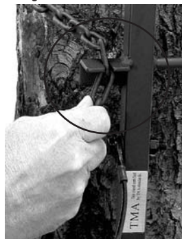
FIGURE 7 INSERT CHAIN INTO SLOTTED CHAIN PLATE
