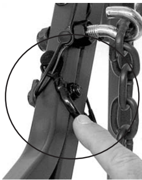
FIGURE 21 PTO PIN INSERTED
