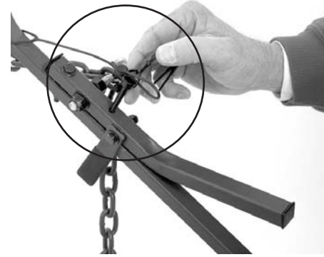
FIGURE 20 INSERT PTO PIN
