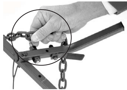
FIGURE 17 SLIP CHAIN OVER EYE-BOLT
