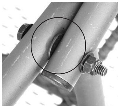
FIGURE 14 NYLON WASHER INSTALLED
